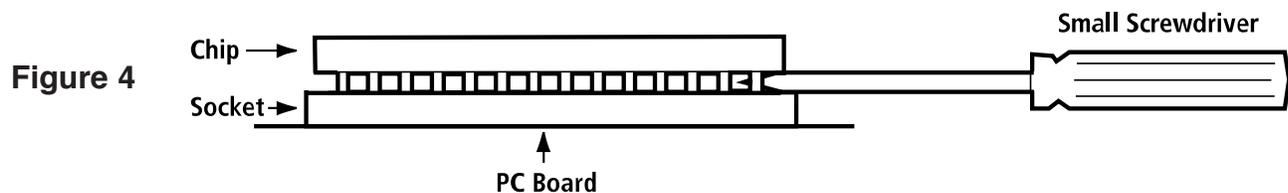
**\*CAUTION:** In rare instances, the referencing slot on the original chip will not be at the same end as the referencing slot in the socket. In these cases, the new performance chip should be installed with the referencing slot in the same position as the original chip.
