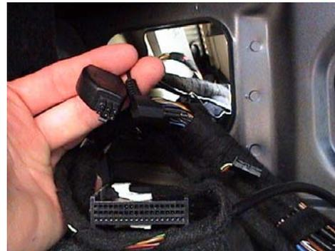
Since the majority of cars have the connector located behind the Drivers Side rear wheel well we will use that as the basis for the remaining photos.
