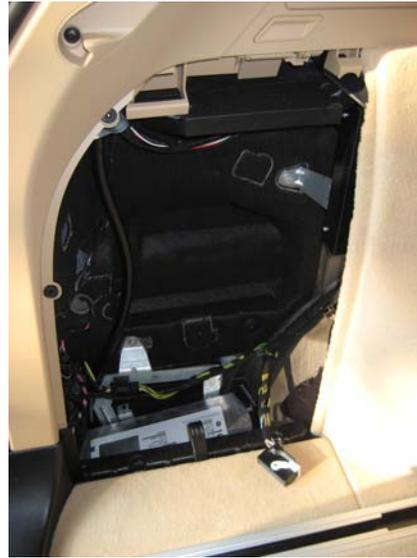
For convertible E46s you will find the connector behind the drivers side back seat seat-back. Access will be via a small silver metal "hatch."
