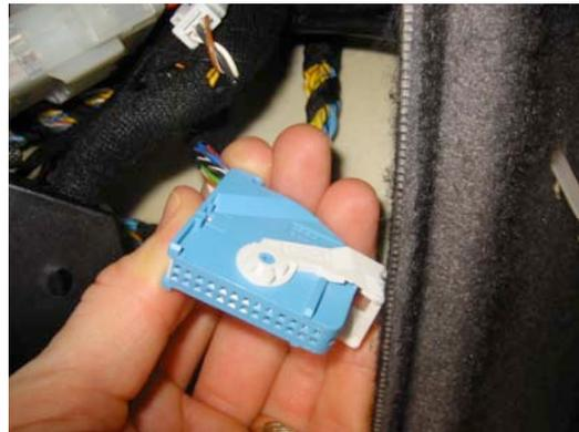
The “SES jumper plug”: This is a blue plug that attaches to the above blue 26pin connector. This plug is necessary for your kit to function. It is BMW part number: 84110018038 and it costs around \$10.00. It may look like this but other versions do exist in BMW warehouses that will work just fine.
