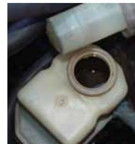
Old, dirty brake fluid inside a brake fluid reservoir.
