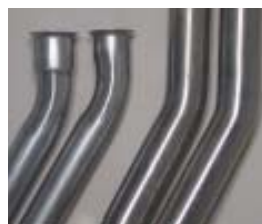
Left: compression bent exhaust pipes collapse in the corners. Right: mandrel-bent Tri-Flo pipes.
