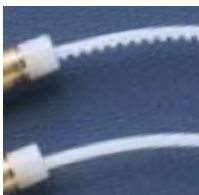
Close-up of nylon retractor cords with teeth (top) and without.
