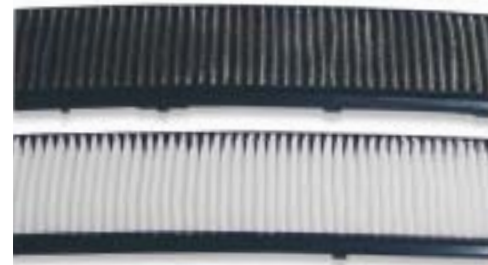
Top: cabin air microfilter from 99 323i after approximately 30,000 miles. Bottom: new cabin air microfilter.
