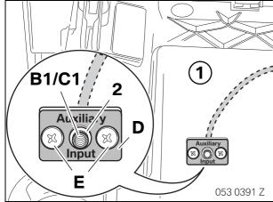
Insert branch **B1/C1** in the glove compartment (1) and secure it to the mounting plate **D** with a knurled nut (2).
