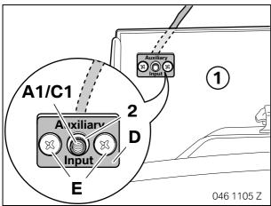
Insert branch **A1/C1** in the glove compartment (1) and secure it to the mounting plate **D** with a knurled nut (2).
